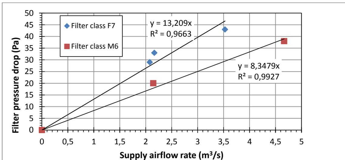
**Figure 22** Filter pressure drop plotted against the supply airflow rate. Data from the field measurements. The pressure increase over the supply air fan with F7 filters installed were: 180 Pa at 0 m<sup>2</sup>/s, 308 Pa at 2,1 m<sup>3</sup>/s and 430 Pa at 3,5 m<sup>3</sup>/s.
