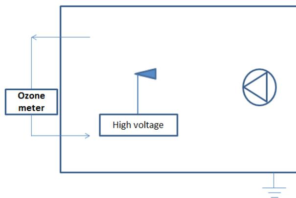
Figure 18 Experimental set-up of the ozone generation test in the test chamber.
