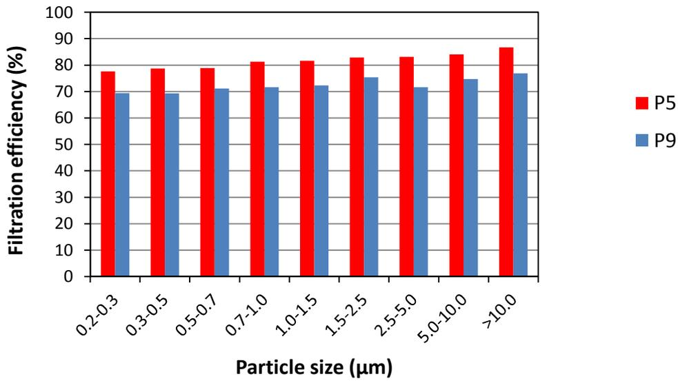
**Figure A2** Filtration efficiency with ionizer assisted on new filter media of P5 and P9.
