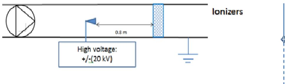
**Figure 15** Experimental set-up of full scale filter test on the G4 class and M6 class filters. The distance between ionizer and filter was 0.8 m for the G4 filter (marked in the figure) and 2 m for the M6 filter.
