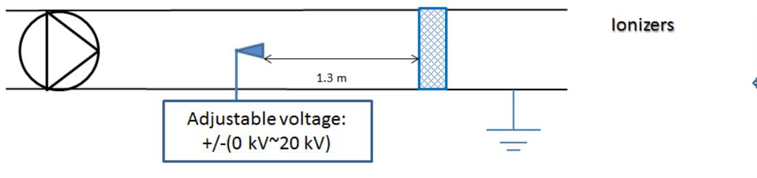
**Figure 8** Experimental set-up of optimum voltage test.
