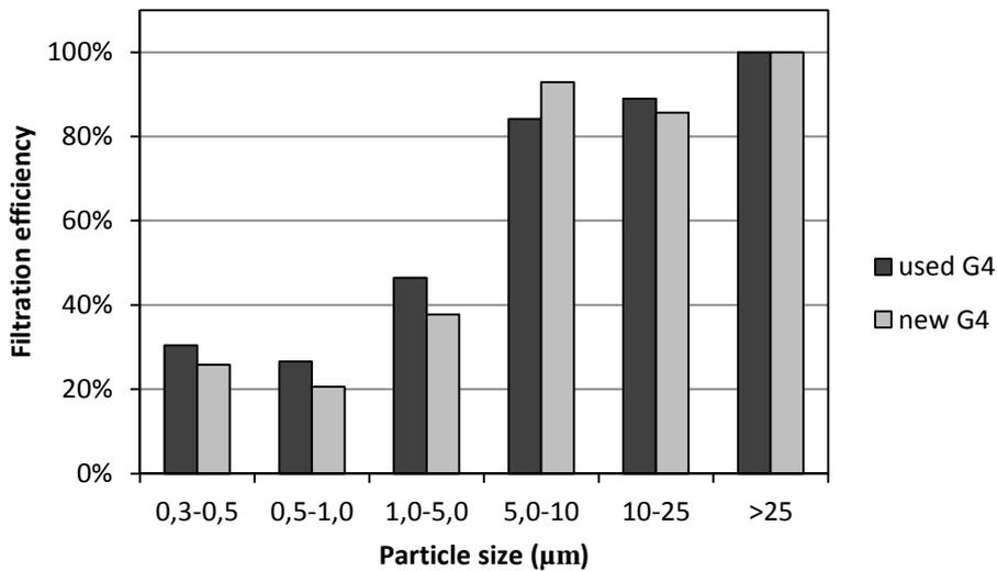
Figure 17 Filtration efficiency of ionizer-assisted full-scale G4 filter produced in the factory. The air velocity through filter media of 0.24 m/s.
