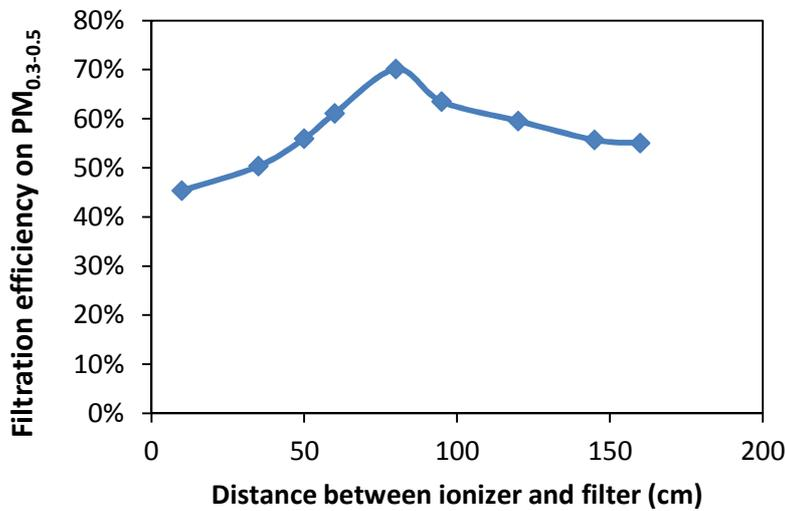
**Figure 7** Optimum distance of the G4 class filters at the upstream particle concentration of  $1 \cdot 10^7$  pc/m<sup>3</sup> and the air velocity of 0.24 m/s through filter media.
