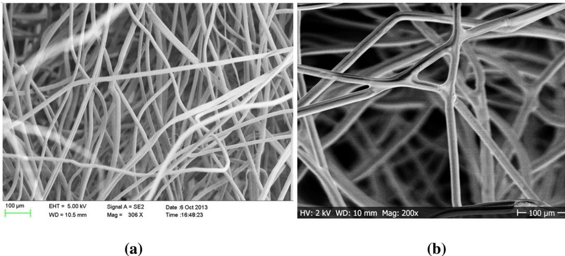
**Figure 2.** Scanning Electron Microscopy (SEM) images of the filter media of (a) M6 class filter; (b) G4 class filter.
