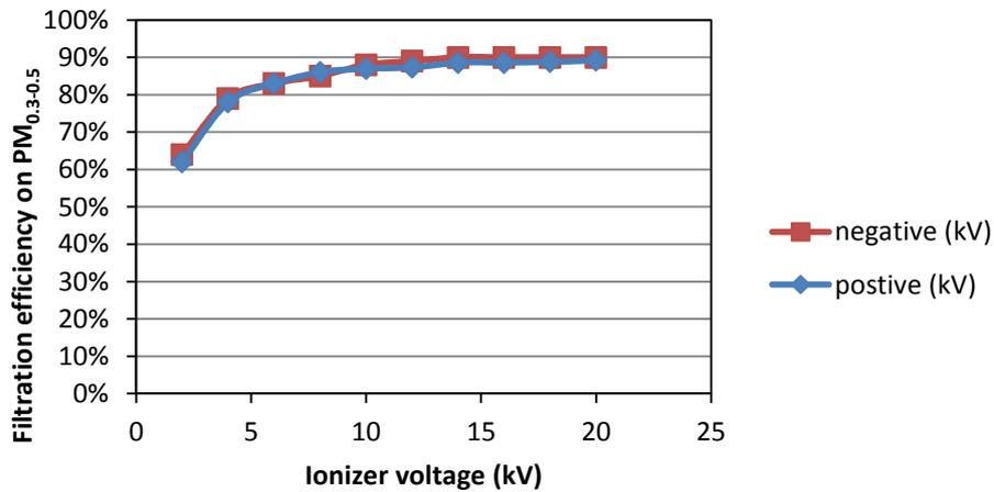
**Figure 9** Filtration efficiency of the M6 class filter when the ionizer voltage was varied from +/-2 kV to +/-20 kV.
