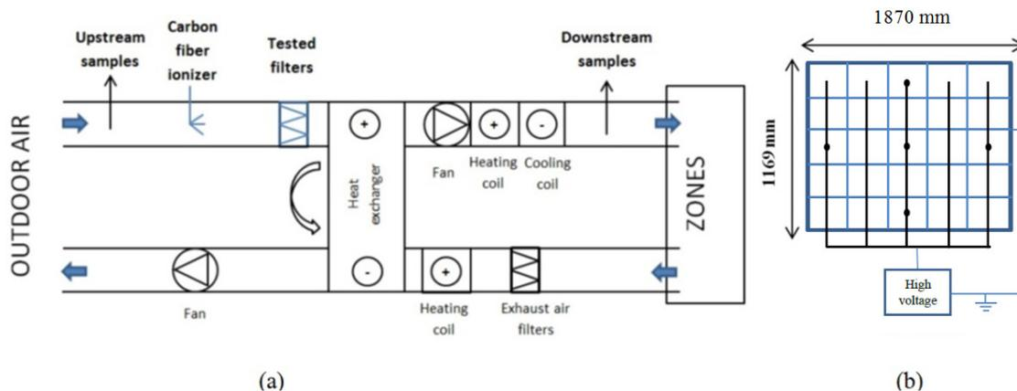
**Figure 20** Sketch of the air handling unit showing the locations of ionization, filters and air sampling. The supply air unit is located below the extract air unit.
