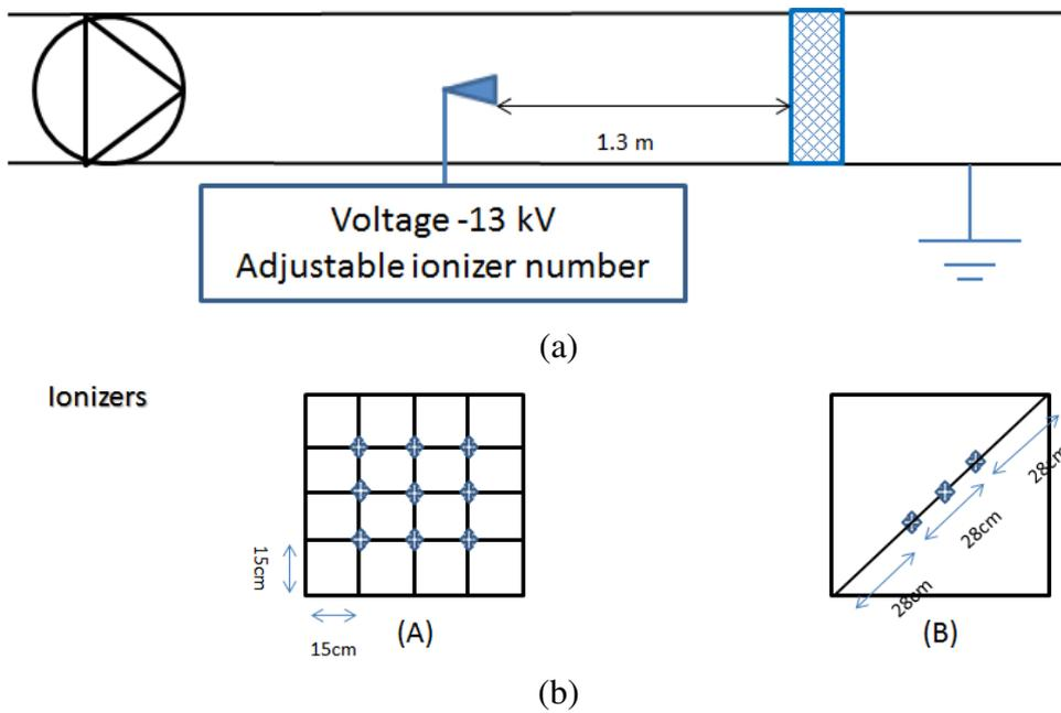
**Figure 11** Experimental set-up of optimum ionizer number and distribution. (a) test rig; (b) ionizer design A and B.
