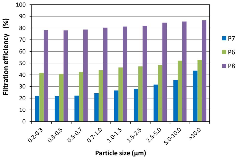
**Figure A3** Filtration efficiency with ionizer assisted on new filter media of P6-P8.
