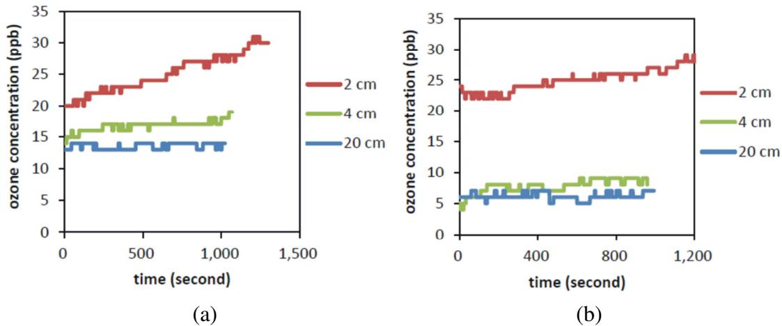
**Figure 19** Ozone concentration in the laboratory test chamber when the distance between the ionizer and chamber wall was 2 cm, 4 cm and 20 cm. (a) negative ionizer; (b) positive ionizer. The ionization voltage was 24 kV.
