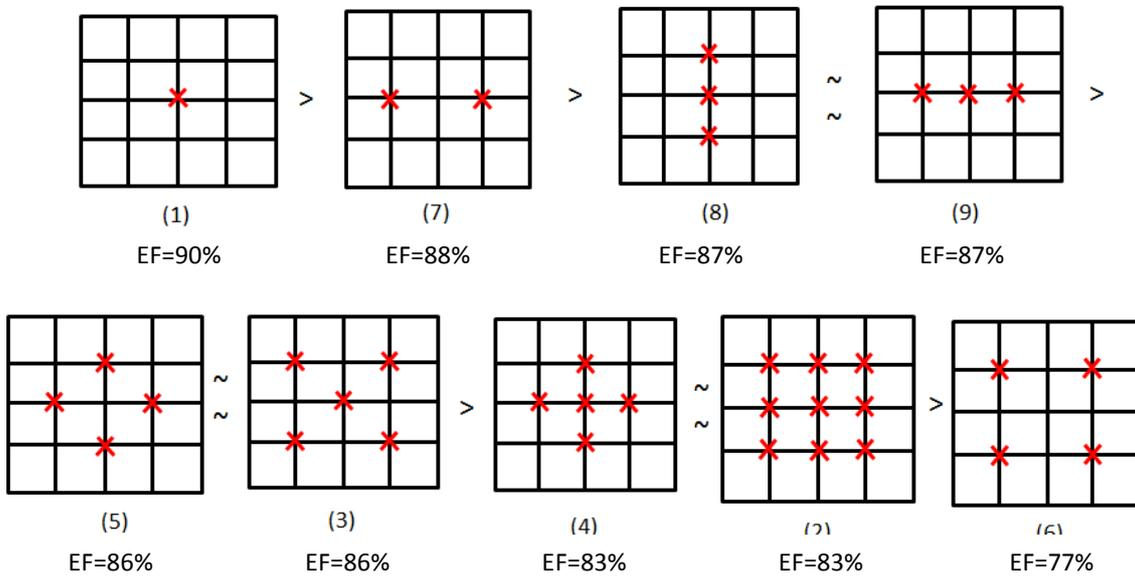
**Figure 13** Ionizer design A. Cases sorted from high to low filtration efficiency for  $PM_{0.3-0.5}$ .
