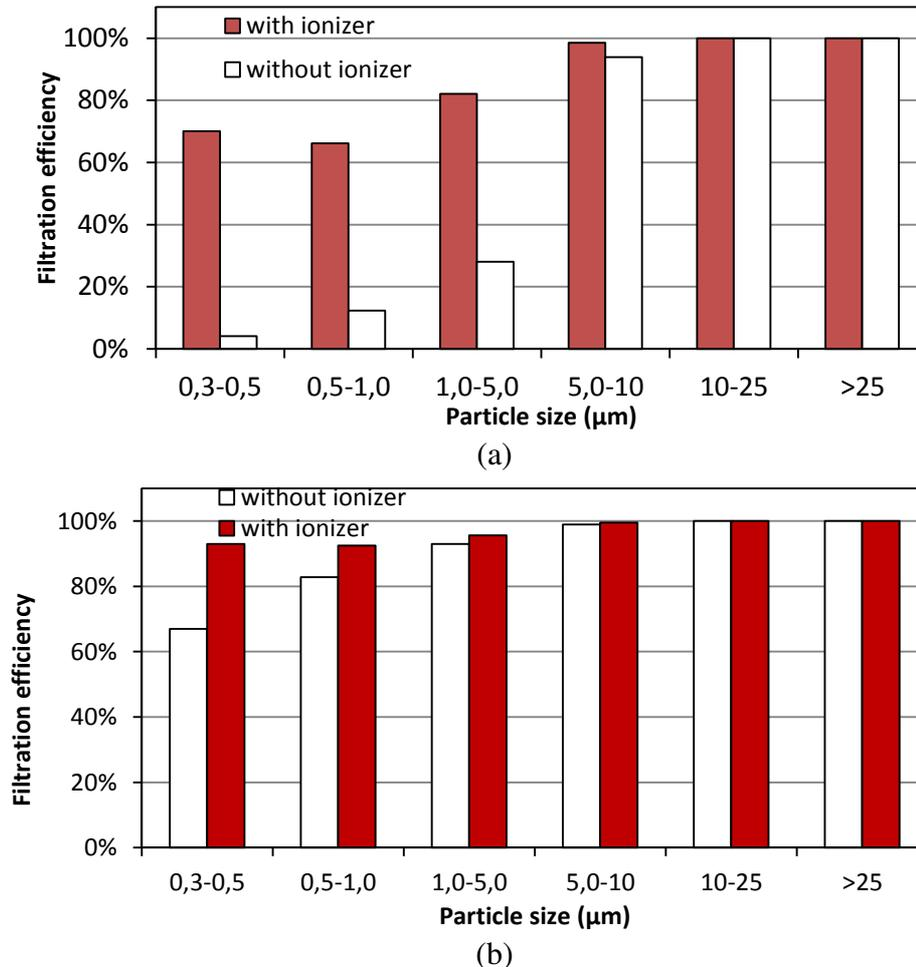
**Figure 16** Filtration efficiency at an air velocity of 0.24 m/s through the filter media (a) G4 class filter; (b) M6 class filter.
