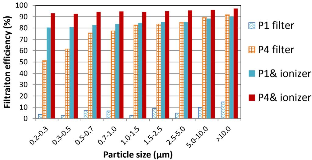
**Figure 4.** Filtration efficiency measured for the P1 (G4 class) and P4 (M6 class) filters tested with and without ionizer. Small scale testing of flat sheets of filter material.
