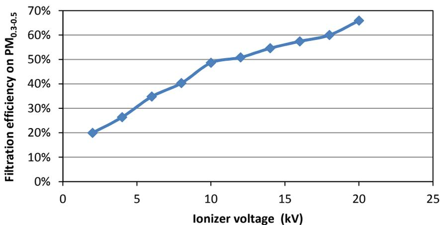
**Figure 10** Filtration efficiency of the G4 class filter when ionizer voltage was varied in the range 2 ~20 kV.
