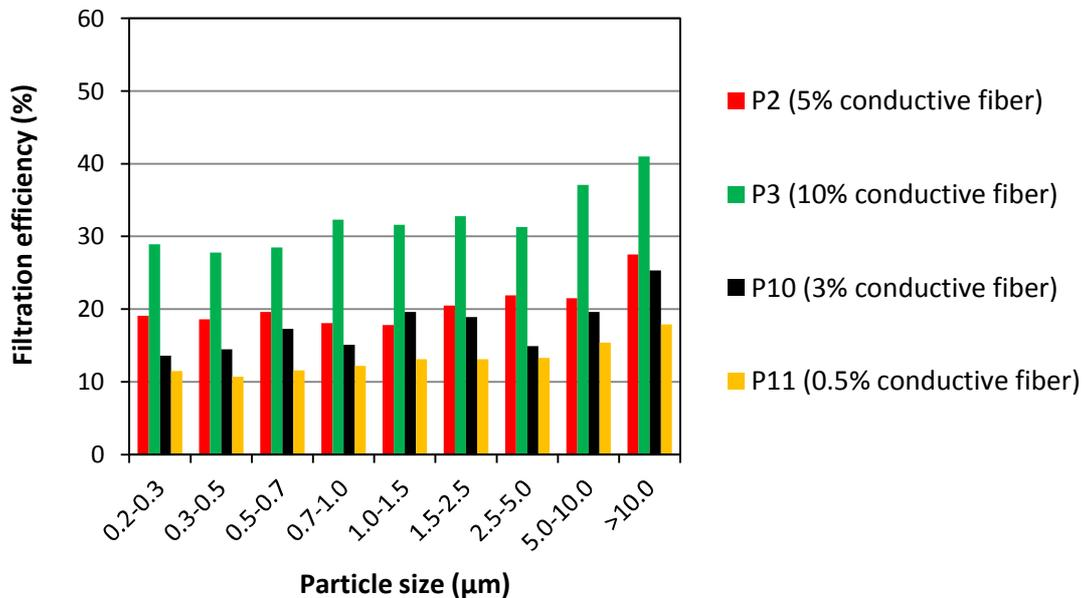
**Figure A1** Filtration efficiency of the filter media assisted with ionizers. These filters consisted polyester fiber and X% conductive fiber.
