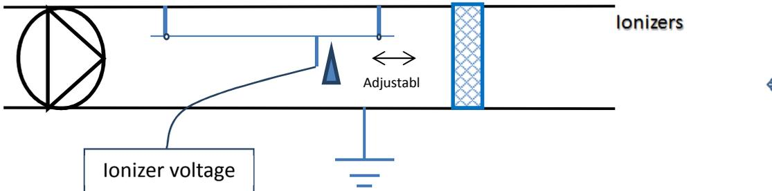
**Figure 5** Experimental set-up of optimum distance test carried out in the full-scale test rig (duct cross section area 0,36 m<sup>2</sup>).
