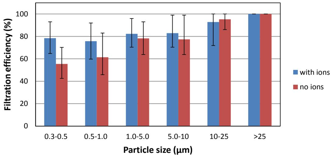
**Figure 21** Average filtration efficiency of M6 class filter during 6 months. The error bars represent the initial (highest) and final (lowest) efficiency within this period. The air flow rate was about 2.2 m<sup>3</sup>/s and the filter cross section area was 2.2 m<sup>2</sup>.
