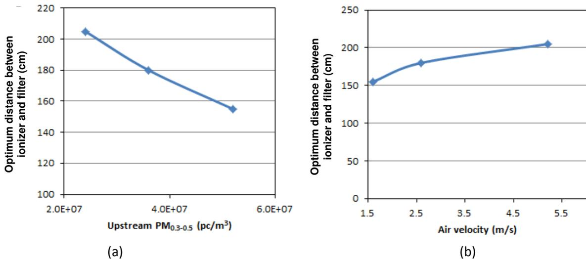
**Figure 6** Optimum distance of the M6 class filters with (a) varied upstream particle concentration at an air velocity of 1.6 m/s (0.2 m/s through the filter medium); and (b) varied air velocity at particle concentration of  $5.8 \cdot 10^7$  particles per m<sup>3</sup> (pc/m<sup>3</sup>).
