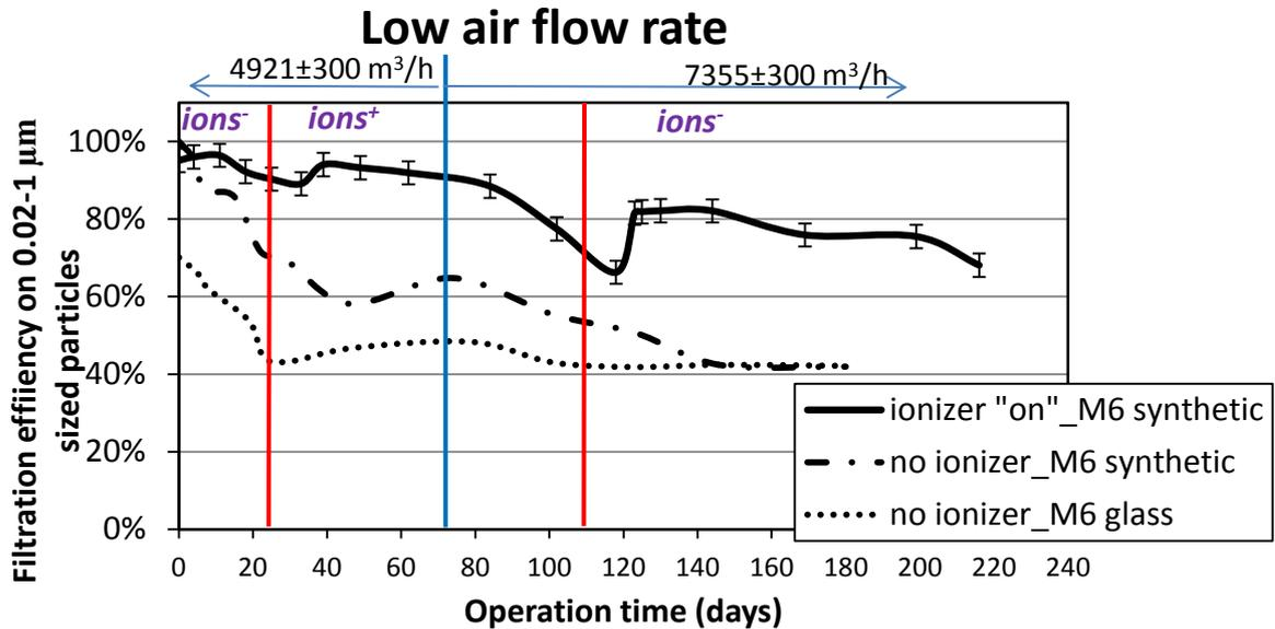
**Figure A1.** Filtration efficiency values (0.01-1 $\mu$ m) measured for the synthetic M6 filter tested in the field with ionization, together with values measured for an identical synthetic M6 filter and a glass fiber filter of class M6 tested in the laboratory without ionization. The data were collected at relatively low air flow rates. The laboratory tests were conducted at an air velocity of 1 m/s, while the field measurements were made at velocities between 0.8 and 1.2 m/s.
