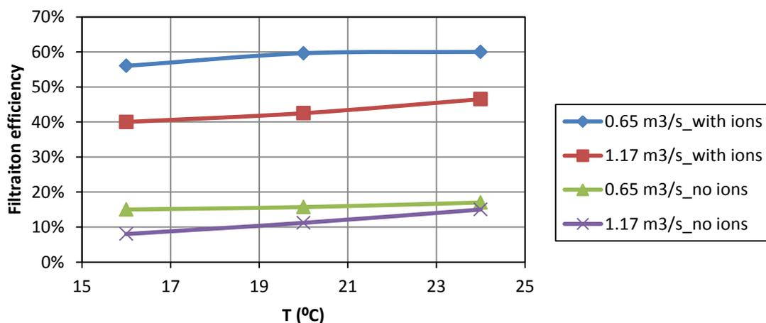
**Figure 11.** Filtration efficiency ( $0.4\mu\text{m}$ ) of the synthetic M6 filter, both with and without ionization, plotted against the upstream air temperature. All data were collected when the filter had been in operation for 6 months.
