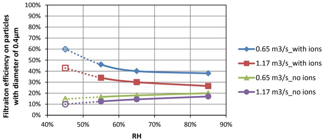
**Figure 10.** Filtration efficiency ( $0.4\mu\text{m}$ ) of the synthetic M6 filter, both with and without ionization, plotted against the upstream relative humidity. All data were collected when the filter had been in operation for 6 months.
