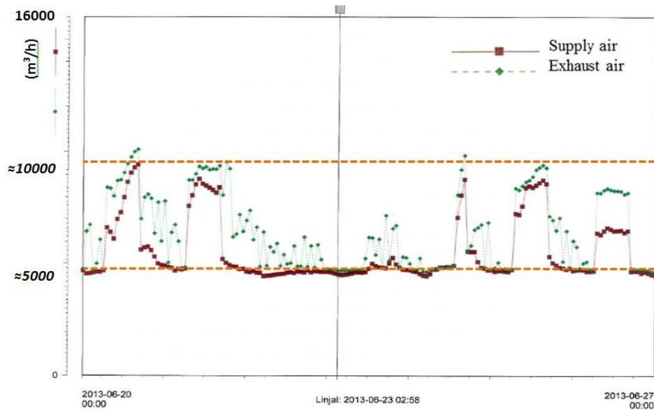
**Figure 2.** Air flow rate in the ventilation system during one week.
