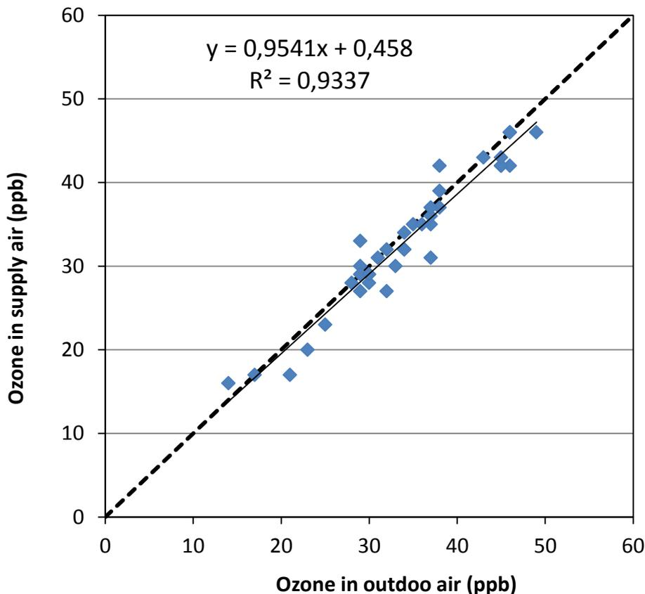
**Figure 9.** Ozone concentrations measured before (outdoor) and after (supply) the ionizer assisted M6 filter tested in the field. The data were collected repeatedly over the entire test period of about 7 months.
