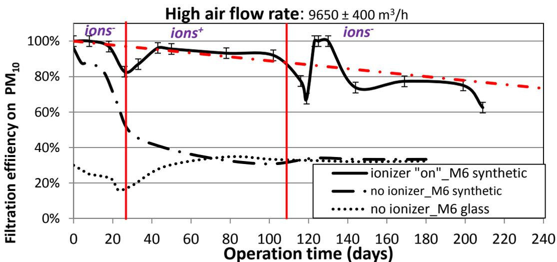
**Figure A4.** Filtration efficiency values ( $\text{PM}_{10}$  mass concentration) measured for the same filters as in Figure A1. The diagram also shows data for a glass fiber filter of class F7, tested in the laboratory without ionization. The data were collected at high airflow rates. Both the laboratory tests and the field measurements were conducted at an air velocity of 1.6 m/s.
