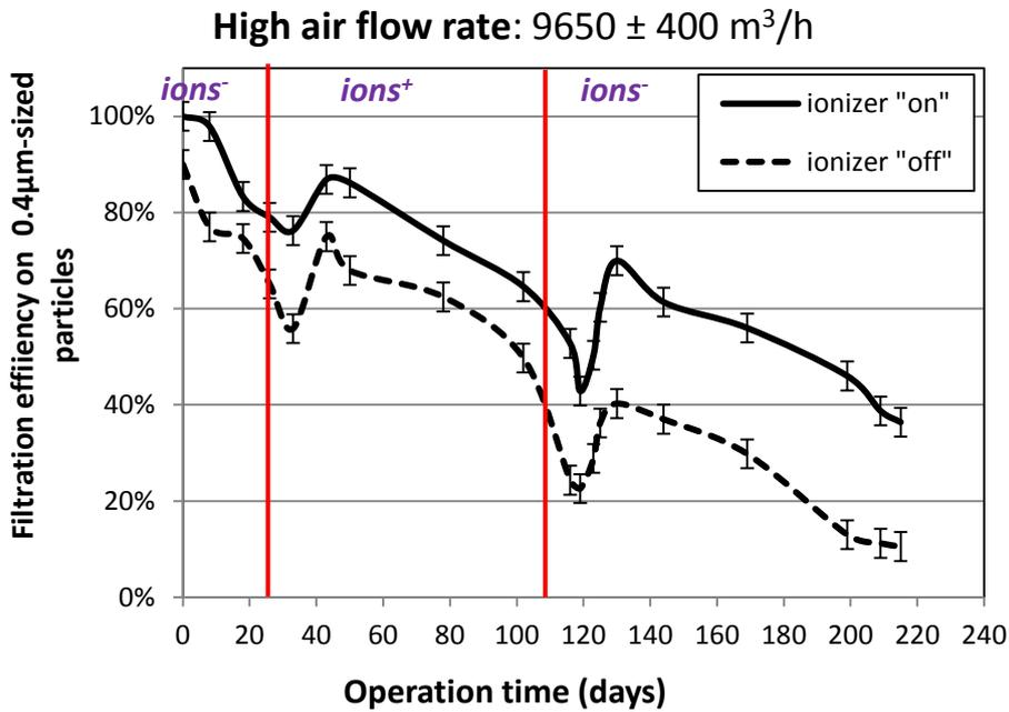
**Figure 4.** Summary of the results from the field measurements. The data were collected when the air handling unit was operating at a high airflow rate.
