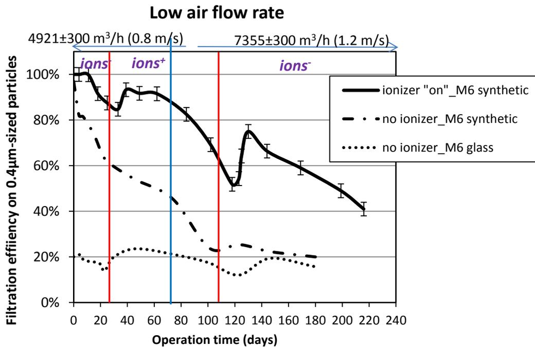
**Figure 6.** Filtration efficiency values measured for the synthetic M6 filter tested in the field with ionization, together with values measured for an identical synthetic M6 filter and a glass fiber filter of class M6 tested in the laboratory without ionization. The data were collected at relatively low air flow rates. The laboratory tests were conducted at an air velocity of 1 m/s, while the field measurements were made at velocities between 0.8 and 1.2 m/s (4920 – 7350 m<sup>3</sup>/h).
