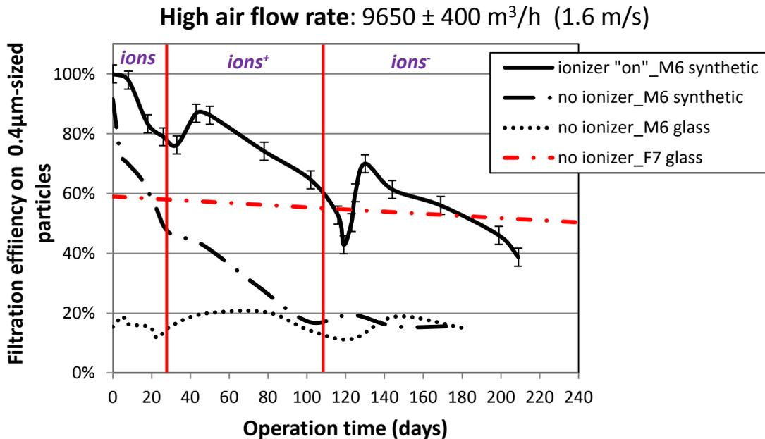
**Figure 7.** Filtration efficiency values measured for the same filters as in Figure 6. The diagram also shows data for a glass fiber filter of class F7, tested in the laboratory without ionization. The data were collected at relatively high airflow rates. Both the laboratory tests and the field measurements were conducted at an air velocity of 1.6 m/s, corresponding to an airflow rate of about  $9650 \text{ m}^3/\text{h}$  in the field air handling unit .
