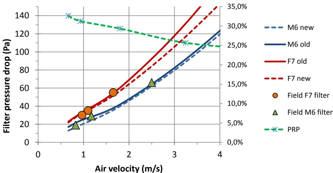
**Figure 8.** Pressure drops measured for the glass fiber filter of class F7 and the synthetic M6 filter together with the pressure drop reduction percentage. The reported pressure drops are the values measured when the filters were new and the values measured after about 7 months of operation. Data from the field test of the glass fiber F7 filter and the ionizer assisted synthetic M6 filter are also presented.
