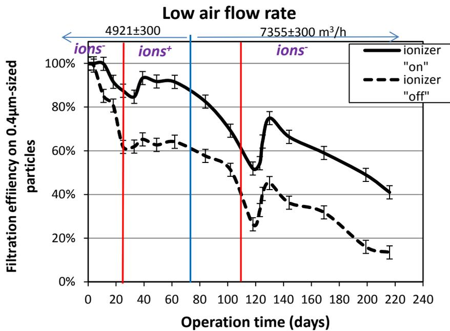
**Figure 5.** Summary of the results from the field measurements. The data were collected when the air handling unit was operating at low airflow rates.
