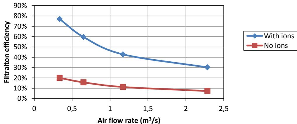
**Figure 13.** Filtration efficiency ( $0.4\mu\text{m}$ ) of the synthetic M6 filter, both with and without ionization, plotted against the supply airflow rate through the filter. All data were collected when the filter had been in operation for 6 months.
