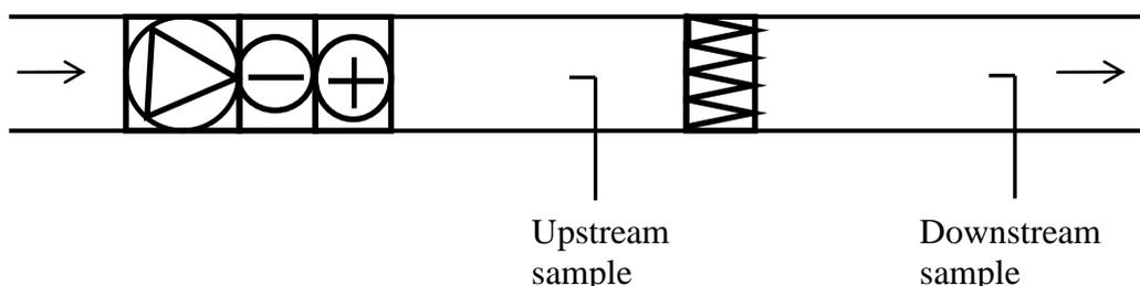
**Figure 3.** Sketch of the laboratory filter test rig. The test rig has room for one filter module of the dimensions 0.6 m · 0.6 m.
