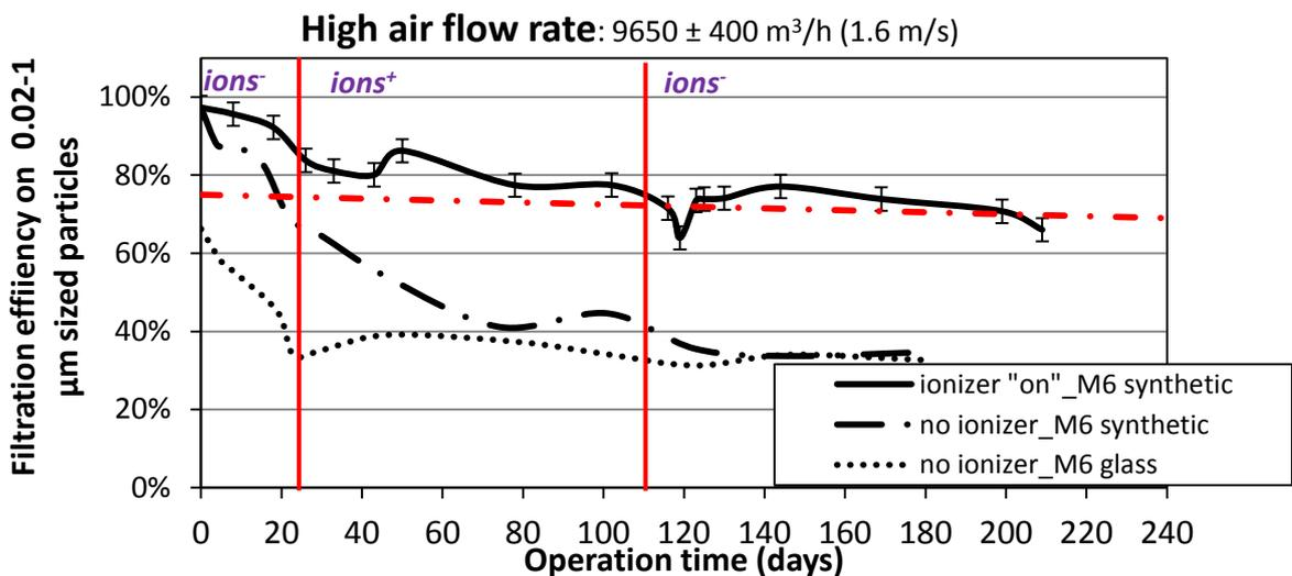
**Figure A2.** Filtration efficiency values (0.02-1  $\mu$ m) measured for the same filters as in Figure A1. The diagram also shows data for a glass fiber filter of class F7, tested in the laboratory without ionization. The data were collected at high airflow rates. Both the laboratory tests and the field measurements were conducted at an air velocity of 1.6 m/s.
