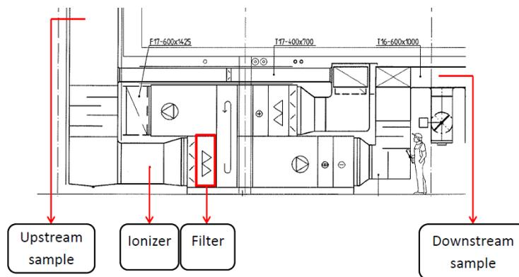
**Figure 1.** Sketch of the air handling unit showing the locations of ionization, filters and air sampling. The supply air unit is located below the extract air unit.
