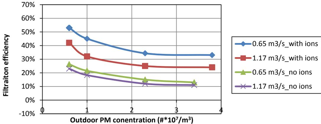
**Figure 12.** Filtration efficiency ( $0.4\mu\text{m}$ ) of the synthetic M6 filter, both with and without ionization, plotted against the upstream concentration of  $0.4\mu\text{m}$  particles. All data were collected when the filter had been in operation for 6 months.
